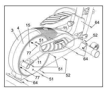
Next, remove the four Screws (51) from the right Pedal Disc (15), and slide the Pedal Disc off. Remove all Screws (52, 64) from the Right Side Shield (4) and the two Bolts (77) from beneath the Pedal Disc, and remove the Right Side Shield (4). Remove all Screws (52) from the Left Side Shield (3) and remove the Left Side Shield.
